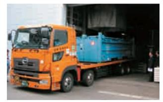
Effluent and sludge transport truck
