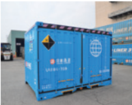
A 12-foot hybrid container that can be loaded onto rail cars and coastal vessels
